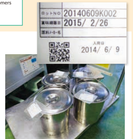
Management through QR code Labels with QR codes are pasted onto all raw materials. All processes, from the receipt of raw materials to production and shipping, are managed through the traceability system using the QR codes.
