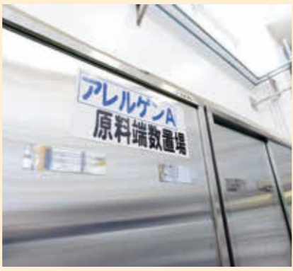
Switching from stickers to stainless steel plates
